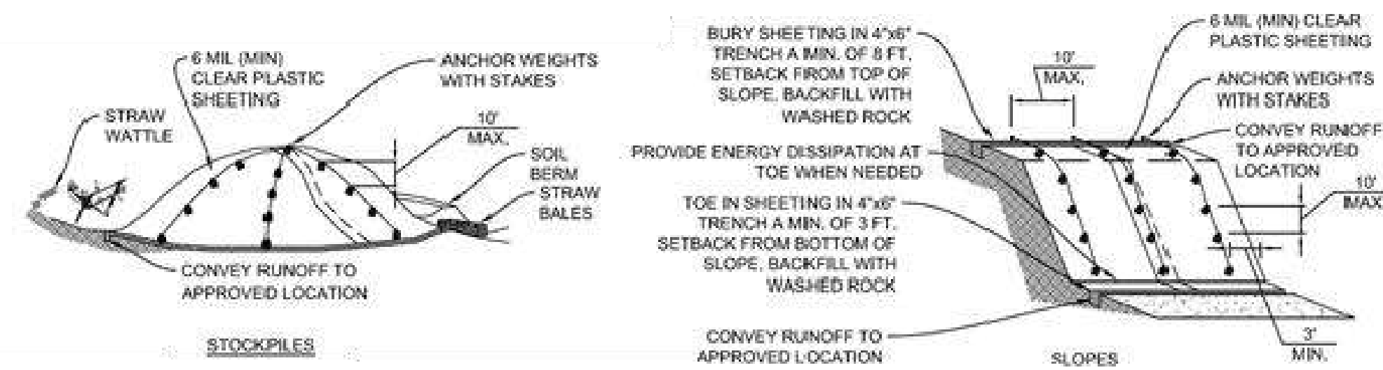
STOCKPILE AND EXPOSED SLOPE COVERING
